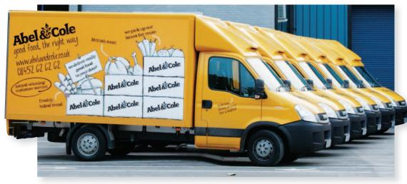
Following its change of spec for 3.5 tonne home delivery vehicles from refrigerated van conversions to refrigerated box bodies, Abel & Cole has ordered 45 more of the new specification vehicles.
